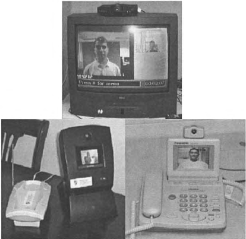
FIGURE 11.5 POTS-based video telephony systems (common types are (a) set-tops, (b) desktops, and (c) all-in-ones. Using low-cost sensors and home automation devices, a living space can easily be retrofitted to collect information about at-home users and their interactions with their environment for health monitoring purposes.
