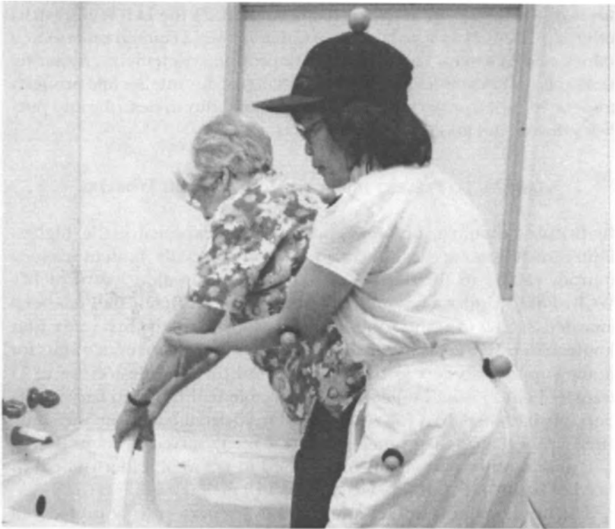
FIGURE 14.1 Transfer aid study of an in-home patient transfer. A home support worker is executing a bathtub transfer with a trained senior aged client in the “transfer aid study.” The round reflector balls (markers) are placed on participants’ selected joints, allowing researchers to estimate risk of injury using the 3-D biomechanical motion analysis system and appropriate biomechanical calculations.
